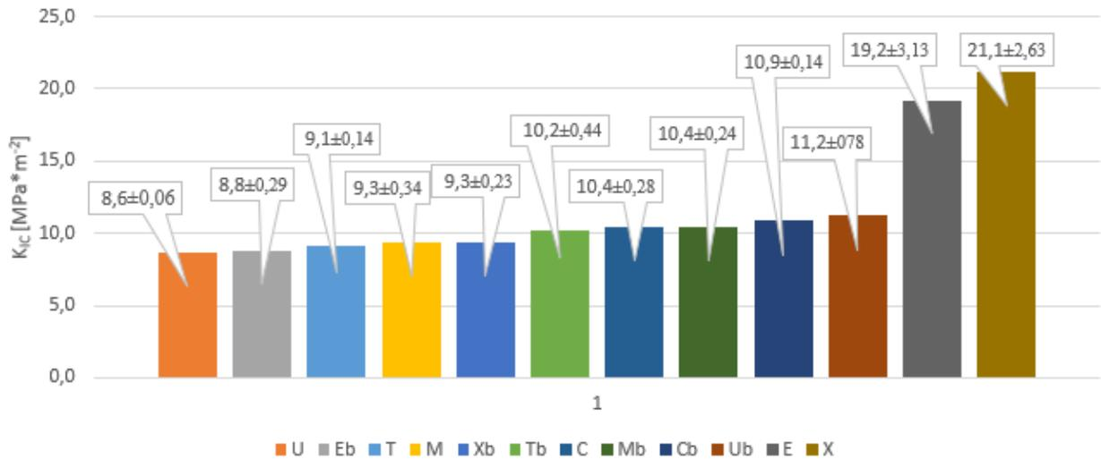
Fig. 5. The impact of boriding on the surface fracture toughness of different types of cemented carbides. The subscript (b) indicates borided samples.
