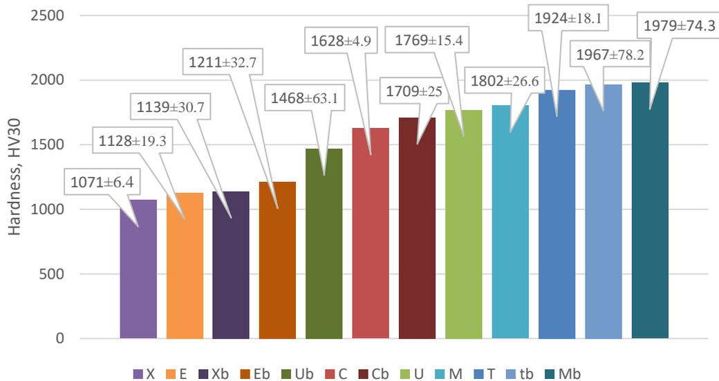
Fig. 4. The impact of boriding on the surface hardness of different types of cemented carbides. The subscript (b) indicates borided samples.
