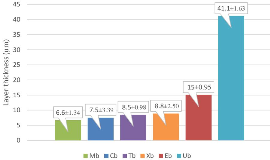
Fig. 2. Thickness of the diffusion layer in the different CCs. The thickness of the diffusion layer was measured on the transverse metallographic section, see Fig. 1.
