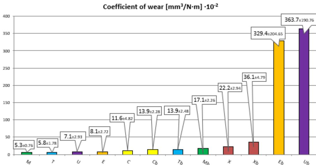
Fig. 6. Effect of boriding on the resistance of cemented carbide to contact loading. In this graph, contact loading is expressed in terms of the wear coefficient. The subscript (b) indicates borided samples.
