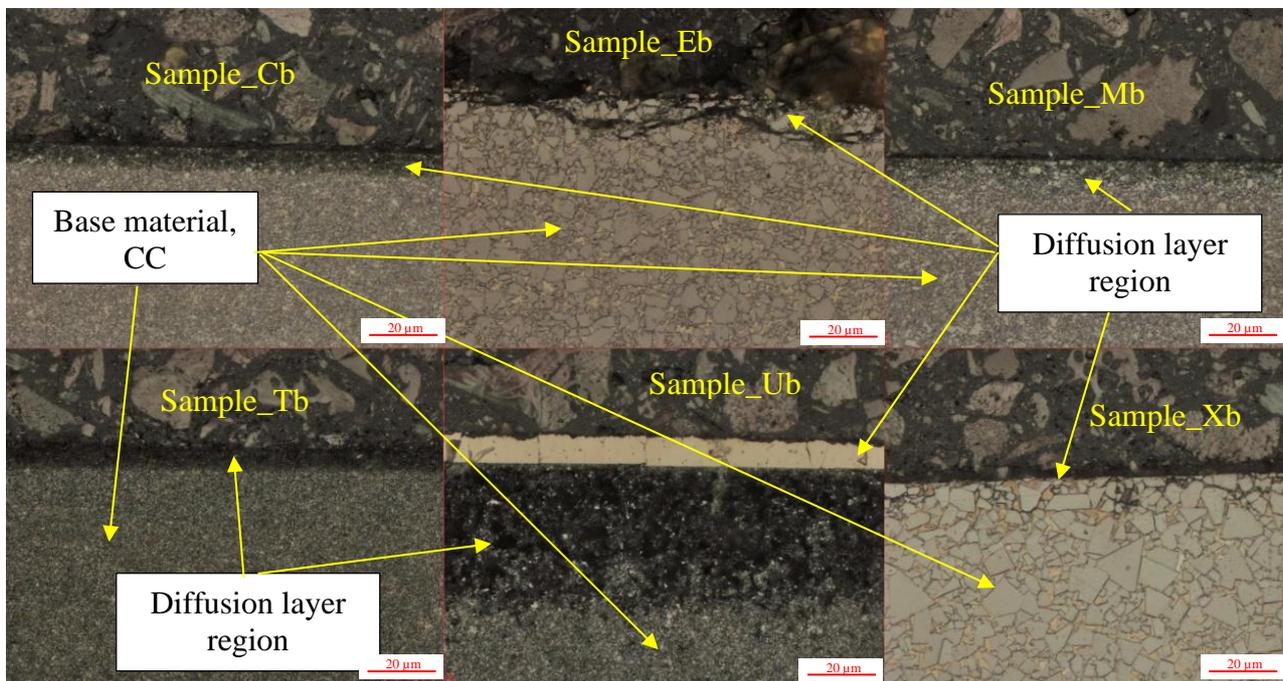
Fig. 1. Transverse metallographic sections through borided CC samples. The subscript (b) indicates borided samples.
