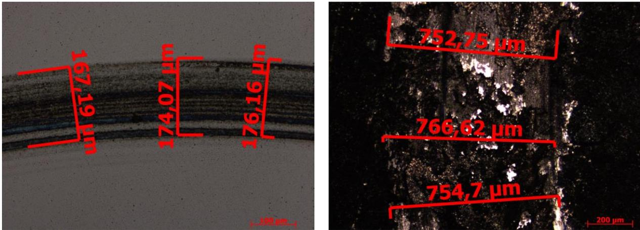
Fig. 7. On the left, there is a portion of a wear track in specimen C prior to boriding; on the right there is a wear track after boriding. In the first case, only abrasive wear was involved, whereas in the second case, abrasive wear was combined with appreciable adhesive wear.
