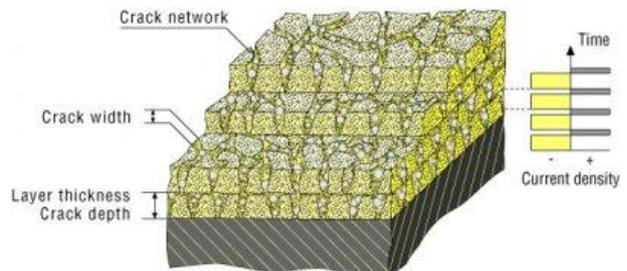
**Fig. 2** Scheme of Cr coating reinforced with hard particles (CKS 36 coating Federal Mogul) [6]
