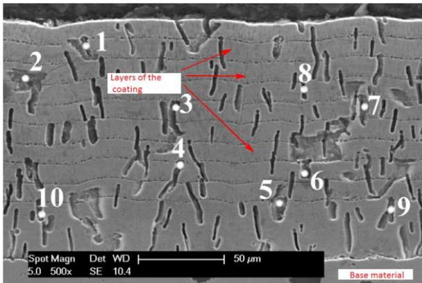
**Fig. 1** Cross section of chromium coating reinforced with  $Al_2O_3$  (BCr coating, Buzuluk a.s.)
