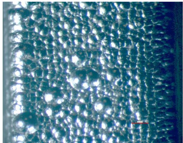
**Fig. 4** Nodules on the surface of hard chromium [8]
